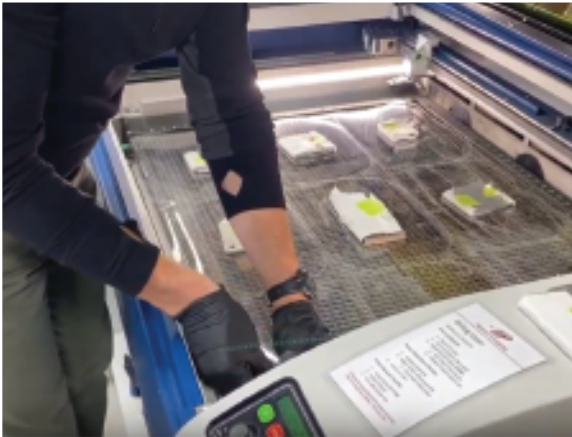
Weigh down each shield to avoid curling. Experiment with speed and power of laser.
