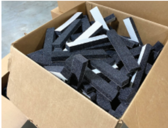
Cut foam to length and width using shear, hot wire, Xacto blade or scissors.
