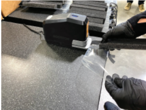
Compress the foam with your thumb to get the elastic to lay flat.Staple the other end of the strap.
