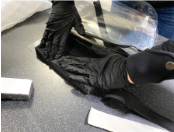
Center foam along top edge of shield and press down to get the adhesive to stick.
