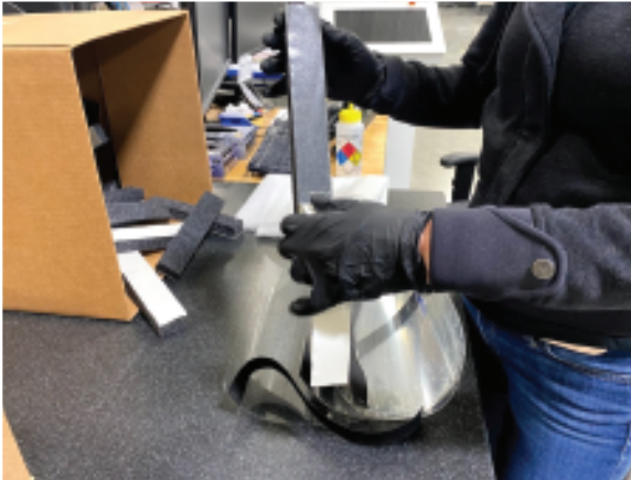
Remove liner from foam to expose the adhesive.
